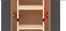
5. Remove the 4x M6 screws that connect the main hinge to the lid.
