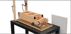
7. Refix the 4x M6 screws that connect the main hinge to the lid starting with the outside predrilled holes first.
