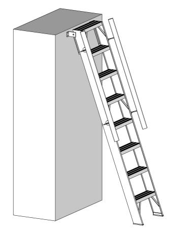
The Sellwood pivotal ladder range are custom built to height as required. When installing the pivotal ladder make sure the ladder feet are flush with the floor level. Fit the pivotal ladder to your fixing point using the timber tight screws supplied.
