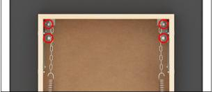
8. Refix the 4x screws that connect the stay arms to the lid using the predrilled holes.
