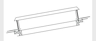
**1.3** The hatch must be flashed in accordance with good roofing practice and using the Metal Roof Code of Practice for detail of flashing.
