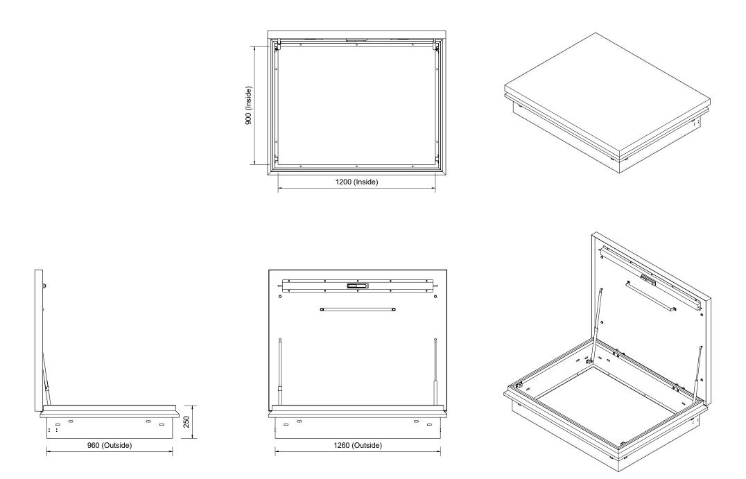
SRH1200900 Roof Hatch | Material: Aluminium | Finish: Powder Coated (Grey)
